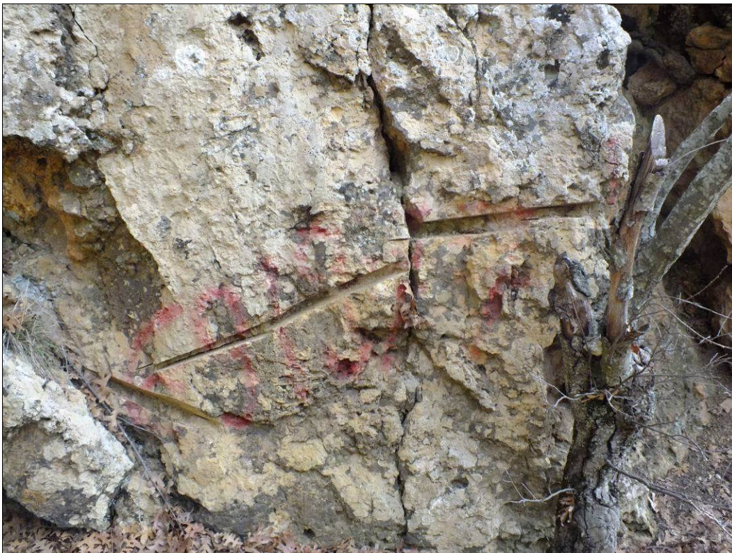
Figure 12.7: Rock-saw channel sampling, eastern Naçak, 471520E 4431835N
