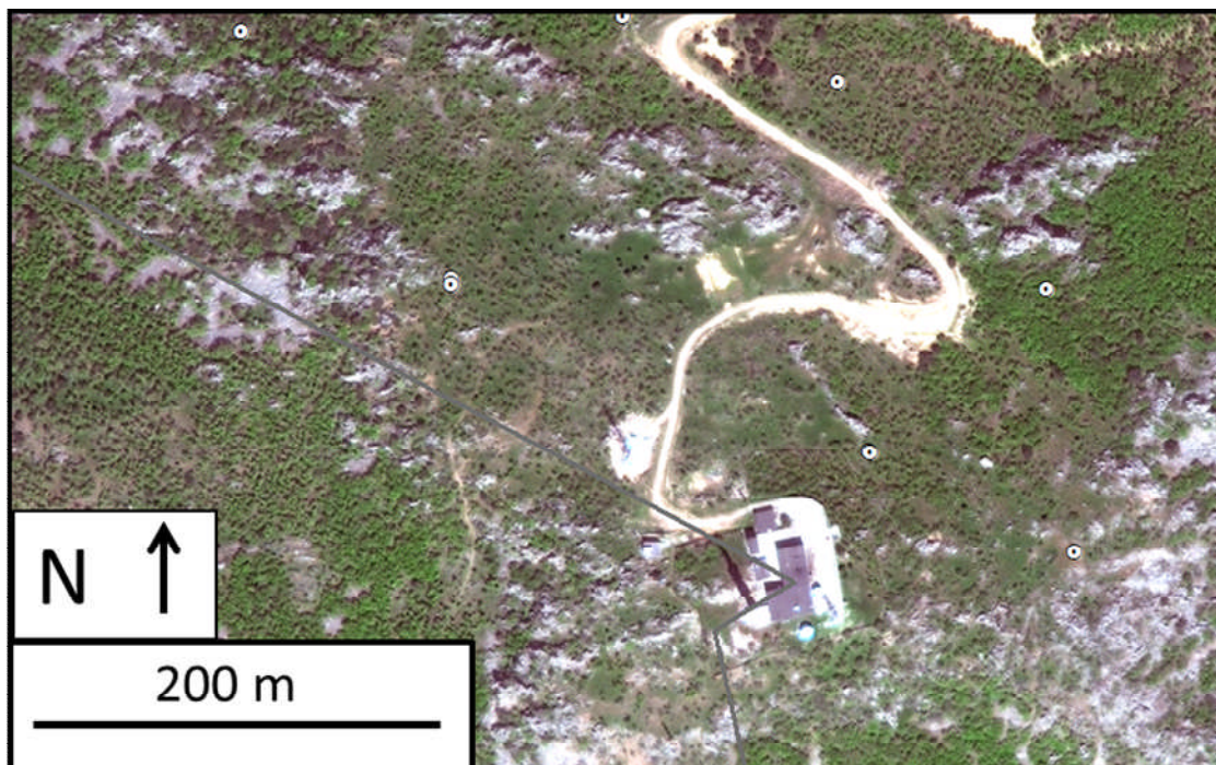
Figure 7.4: Quickbird images showing silica ribs with strong N80E orientation and secondary NW orientation at the Kayalı target.
