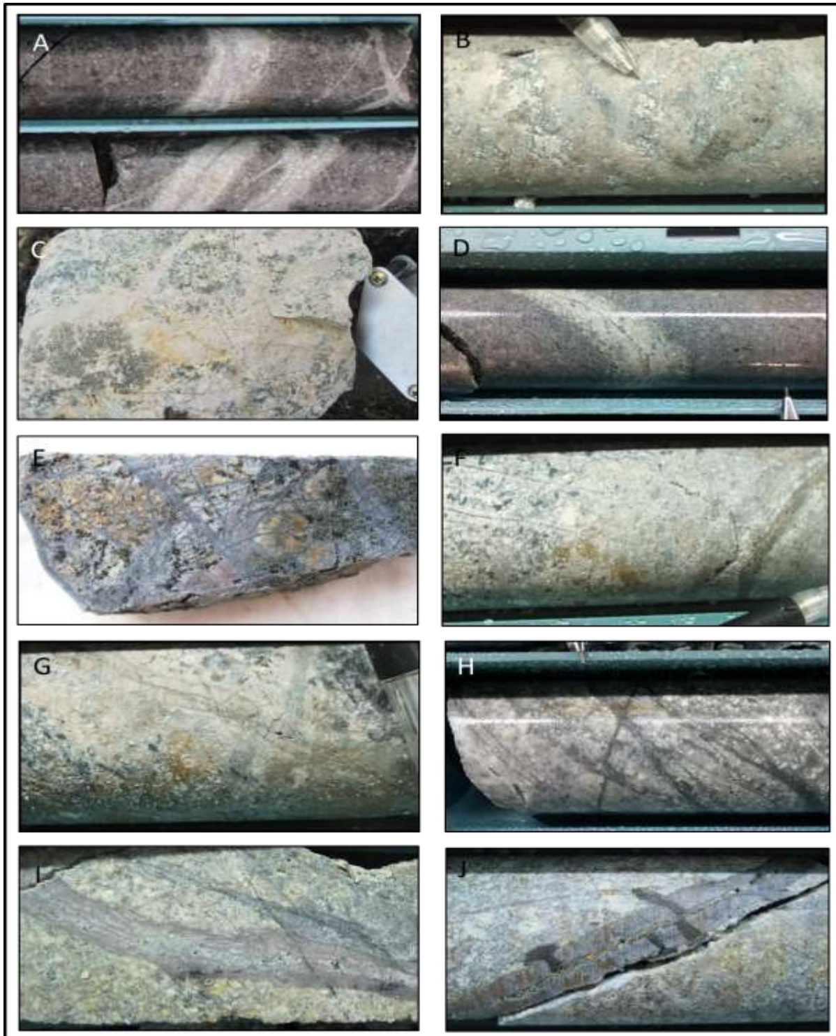
Figure 7.7: Examples of porphyry-related alteration at TV Tower
